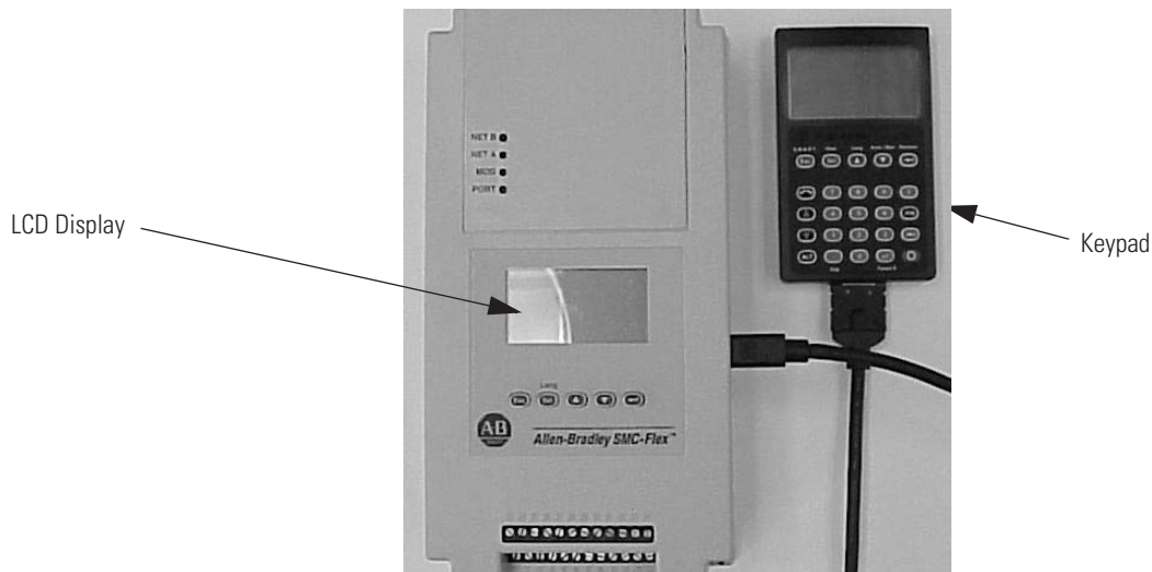
Figure 1.35: LCD Display with Keypad
